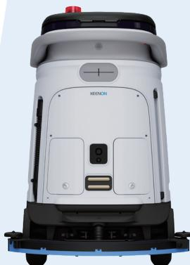
The dual-battery compartments support hot-swapping while powered on, allowing quick replacement in just 5 seconds. This completely breaks away from the inefficient cycle of "2 hours charging, 2 hours operation" common in traditional cleaning machines.
